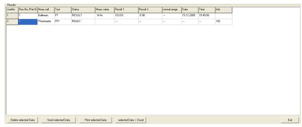
In the field results you see the current conditions of the measurements and the results can read. In order to print results / send results (LIS) / export results to Excel / delete results, mark the according results with the PC mouse before you click on the according button below the results.
