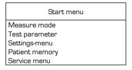
Select "Measure mode" by means of the arrow keys and confirm by pressing the ENTER-key. You have to communicate the MC 4<sup>plus</sup> now in the work mode menu whether a running number or a Pat.-ID shall be used for the sample test result identification.
