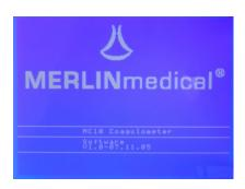
After approx. 15 sec. the display changes automatically from the welcome display to the start menu. The signal lamps do no longer light up.
