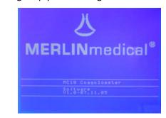
After approx. 15 sec. the display changes automatically from the welcome display to the start menu. The signal lamps do no longer light up.
